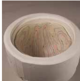
15 The final shaping can be done in a mould where it can be rested to firm up before attaching a rim, handles and foot, if these elements are desired.
