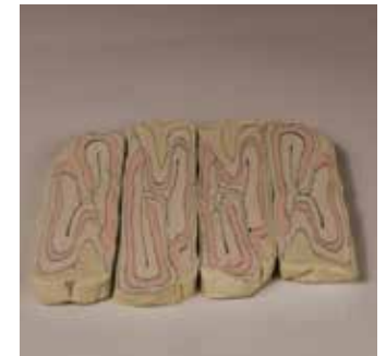
12 Multiple slices are then arranged to make an agreeable design before being brushed with clean water and gently agitated together to adhere and form the pattern slab.
