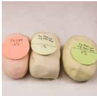
4 The colours used for this vessel are illustrated underneath the fired test tiles. The primary colour ratios and saturation levels are noted on each test tile. As can be seen, fired colours are usually deeper than the raw coloured clay.
